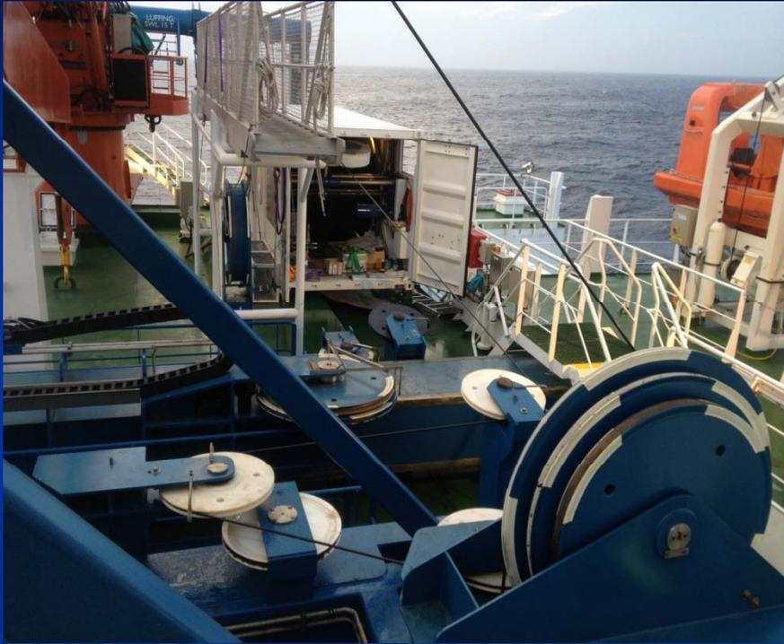
Left hand side view showing the rope run from the container over the Nylatron sheaves for deployment over the starboard forward deployment system.
