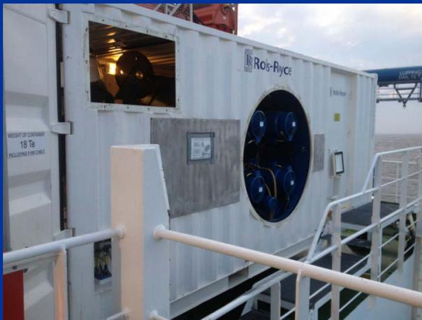
Right hand side view showing the 4 electric motors located inside the drum driving the slew ring.
