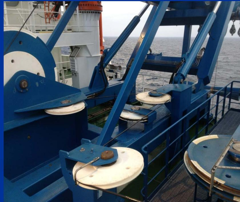
RRS Discovery clean CTD rope sheave run over forward starboard deployment system
